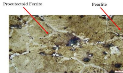
Figure 15. As cast structure (X100)
