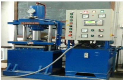
Figure 3. Laminate in compression moulding machine (Courtesy: CEG, Anna University)
