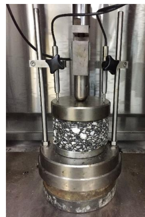
Figure 4. Dynamic creep sample using UTM-5
