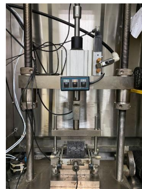
Figure 3. UTM-5 with a resilient modulus test fixture
