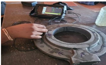
Figure 17. Ultrasonic testing of valve body casting
