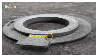
Figure 1. Shrinkage defect in butterfly valve body
