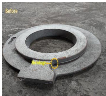
Figure 4. Shrinkage defect in butterfly valve body casting
