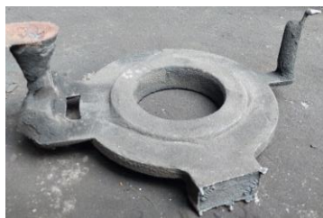
Figure 3. Existing gating system
