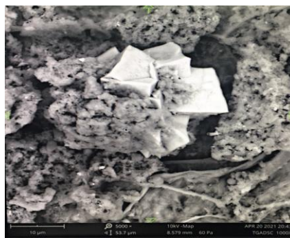
Figure 5. SEM image of finely ground okra mucilage powder at \times 5,000 magnification
