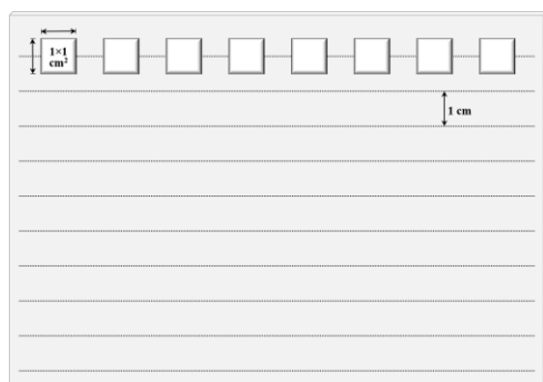
Figure 3. Positions and orientation of hydrogel pads on a clear acrylic substrate. Note that the horizontal lines are on a sheet of paper attached under the substrate
