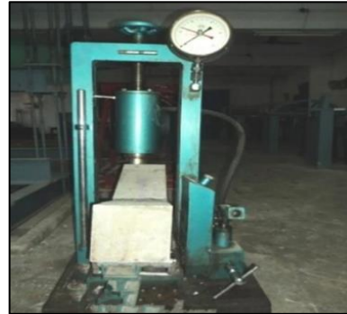
Figure 7. Testing of PCCB
