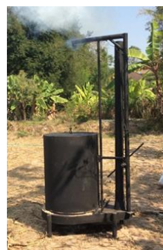
Figure 3. An improved vertical charcoal kiln
