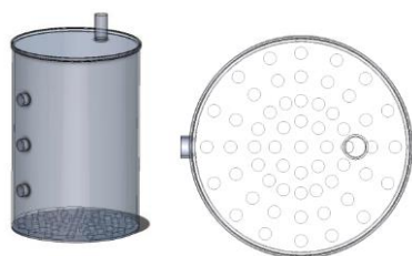
Figure 2. The model of original vertical charcoal kiln in Thailand
