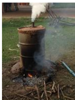
Figure 1. The original vertical charcoal kiln in Thailand
