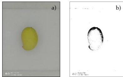
Figure 2. Pre-processing converting original bagged mango image to grey-scale image a) and binary image b)
