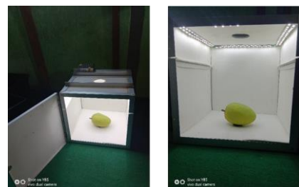
Figure 1. The setup used to capture the images in which the size of light box was 24.13 cm×27.94 cm and light intensity
