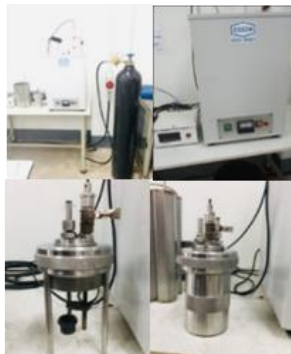
Figure 1. Bomb calorimeter system used in the present study
