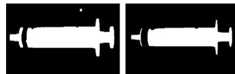
Figure 4. (left) Dilated binary image, (right) Eroded binary image after a dilation
