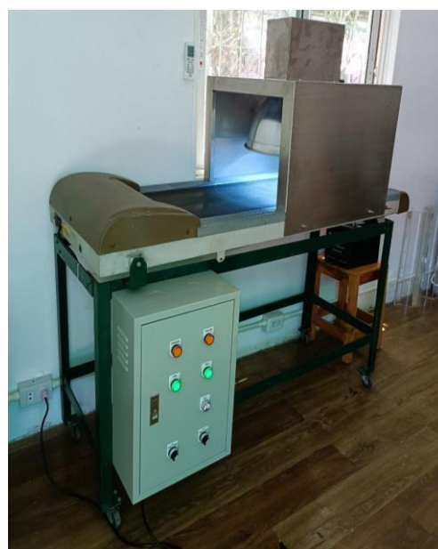
Figure 3. A prototype of a low-heat sterilization system for pulsed light packaging
