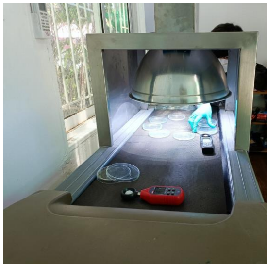
Figure 5. The sterilization test for Escherichia coli bacteria
