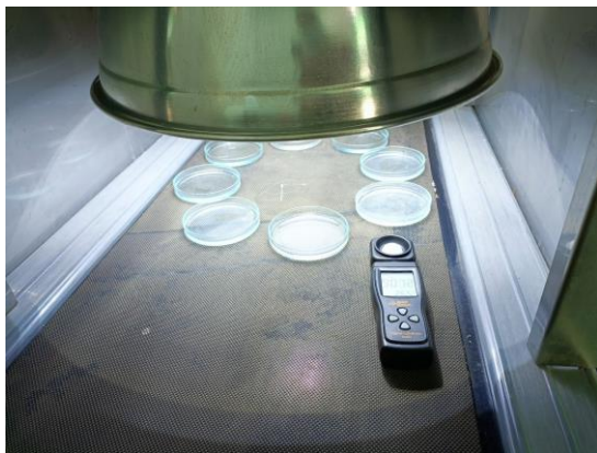
Figure 8. Sterilization test for Bacillus cereus bacteria
