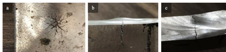
Figure 8. Macro deformation of (a) the back of plate 1, (b) the back of plate 3, and (c) the side of plate 3
