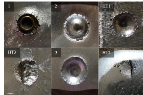
Figure 6. Ballistic resistance mark, from the deepest penetration (upper left) to the most shallow penetration (bottom right)
