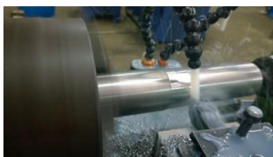
Figure 1. The cutting zone under cooling condition
