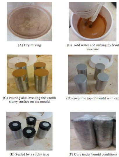
Figure 8. Stage preparation of soil-cement columns.
