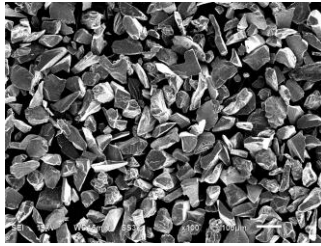
Figure 1. Morphology of the angular silicon carbide particle by SEM
