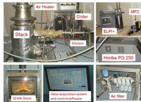
Figure 1. Experimental setup for emission measurements from wood stoves, conducted in a laboratory, Namur, Belgium, PRD = Porous tube diluter, ED = Ejector diluter, MFC = Mass flow controller
