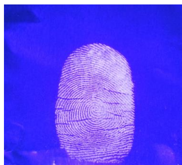
Figure 7. \text{Gd}_2\text{MoB}_2\text{O}_9:\text{Sm}^{3+} on the aluminum foil surface under UV excitation
