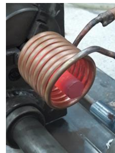
Figure 6. Specimen setup and preheating of specimen by induction heating coil
