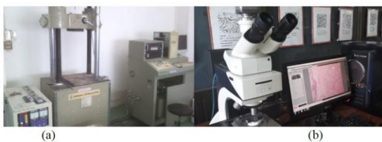
Figure 4. The testing machine: (a) Tensile testing (b) Image analysis
