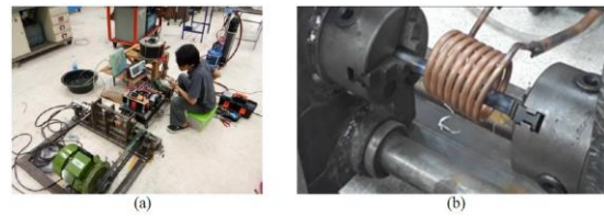
Figure 5. Experimental setup: (a) Friction welding machine (b) Specimen setup
