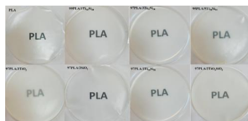
Figure 4. Photographs of films prepared from PLA and PLAnanocomposites (250-300 \mu\text{m} thickness)
