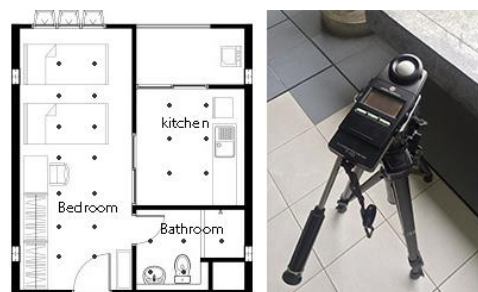
Figure 2. Drawing with measurement points of an investigated area (left) and photograph of instruments (right) in part II in study I
