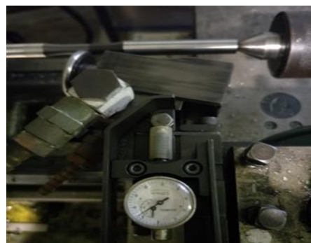
Figure 2. The compressed deep rolling setup
