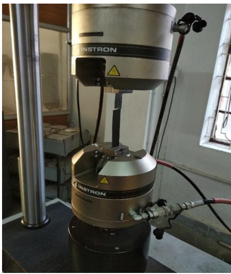
Figure 4. Carbon/epoxy LCB put under tensile test using INSTRON 8862
