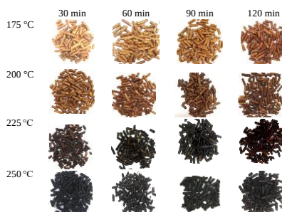
Figure 5. Photograph of the torrefied pellets at different TT and RT; corncobs/cornhusks pellets
