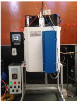
Figure 3. Photograph of the torrefaction chamber
