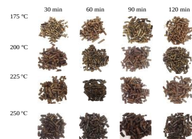
Figure 7. Photograph of the torrefied pellets at different TT and RT; sugarcane trash pellets
