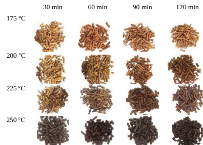
Figure 6. Photograph of the torrefied pellets at TT and RT; rice straw pellets
