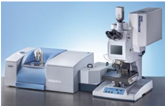
Figure 11. The FT-IR microscopy (Tensor 27 Hyperion)
