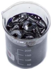
Figure 8. The sliced-XLPE during staining
