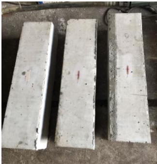
Figure 14. Location of strain gauges on both sides of beam specimens
