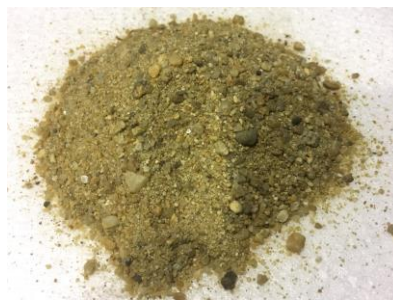
Figure 4. Natural sand used as fine aggregates
