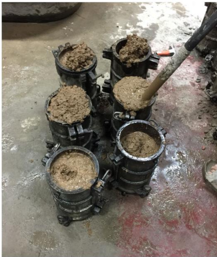
(a) Casting of cylindrical specimens
