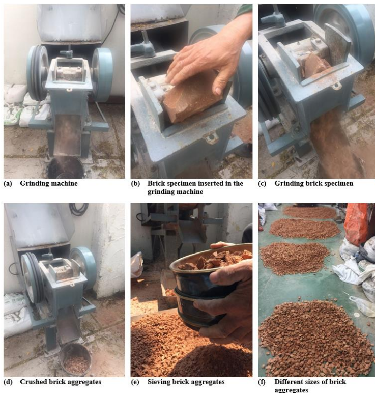
Figure 6. Process of preparing coarse aggregates from fire clay bricks
