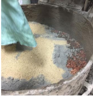
Figure 7. Batching of concrete mix with brick coarse aggregates
