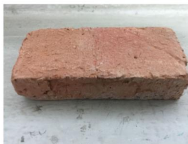
Figure 1. Typical fired clay bricks in Thailand (Thomson Tiles Factory, 2013)
