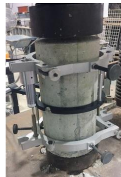
Figure 11. Specimen with extensometer
