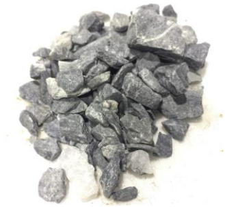
Figure 5. Natural coarse aggregates used for the experimental program
