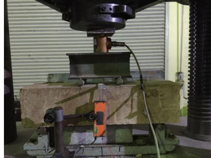
Figure 15. Load setup to test flexural strength of concrete beams
