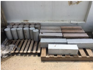
Figure 10. Concrete specimen ready for strength testing after curing
