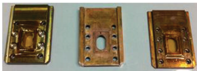
Figure 3. Sample container of cement paste for WAXS analysis
