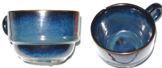
Figure 8. Appearance of the introduced EAFD-bearing glaze (T4) on a cup
