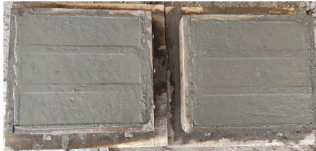
Figure 5. Shows preparation of shrinkage prisms
