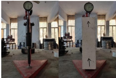
Figure 8. Shows experimental setup for shrinkage measurement
