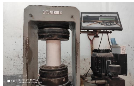
Figure 7. Shows experimental setup for compressive strength test
