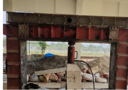
Figure 6. Shows experimental setup for beam load test
