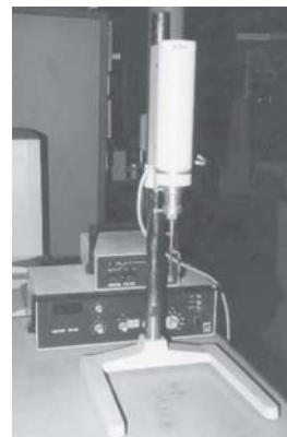
Figure 1. HAAKE rotational viscometers type M 1500
