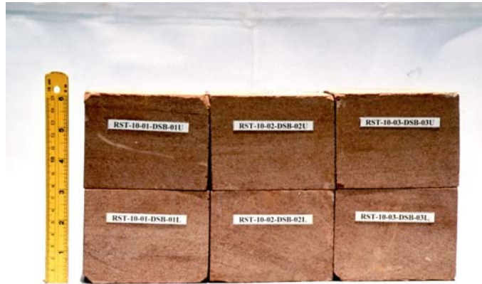
Figure 2. Arkosic feldspathic sandstone block specimens with saw-cut surface prepared for \phi_b determination
