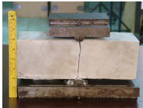
Figure 7. Line load applied on rock block to create tension-induced fracture
