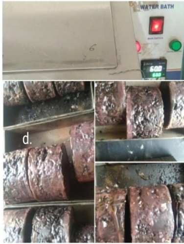
Figure 3. Shows (a) Dimension measurement; (b) oven heating at 60°C, 120 minutes; (c) Marshall test setup; (d) Wax-coated Marshall Specimens in water bath for conditioning at 60°C for 24 hours
