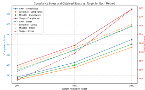
Figure 14. Performance Envelope - Plot of compliance vs weight reduction vs stress limit for all methods
