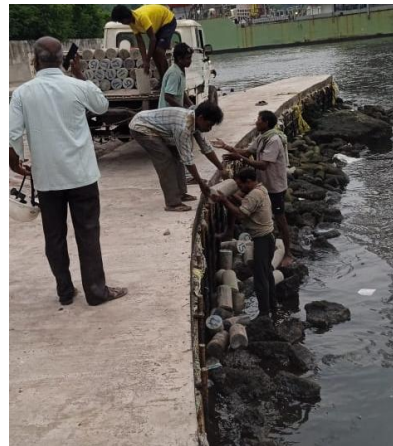
Figure 8. Exposing concrete specimens in a marine environment
