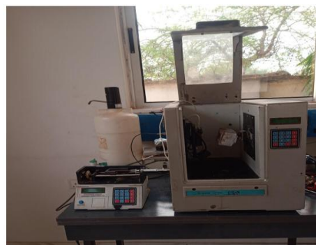
Figure 1. Setup of a Spray Pyrolysis Machine (USP 1500) and Syringe Pump
