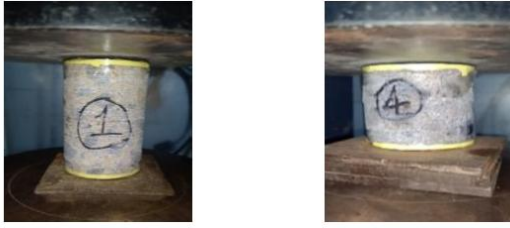
Figure 5. Compressive strength test setup showing cored specimen positioned in the CTM
