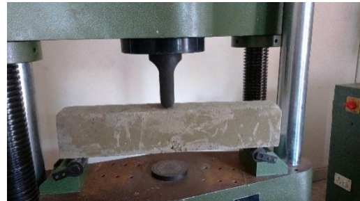
Figure 1. Three-Point Bending Test Setup for Notched Beam Specimens
