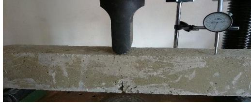
Figure 7. Post-failure photograph of a beam specimen showing crack propagation
