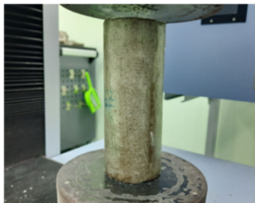
Figure 3. Position of the compression test specimen on the UTM
