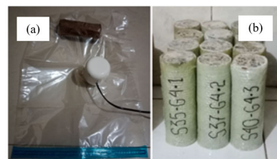
Figure 2. Specimen preparation: (a) vacuum bag, and (b) e-glass skin
