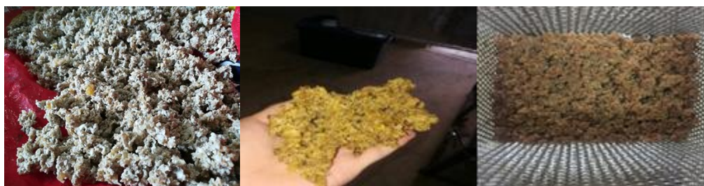
Figure 2. Visual comparison of STR20 physical properties: the top panel shows the raw STR20 sample, while the middle and bottom panels display the cured STR20 sample after drying
