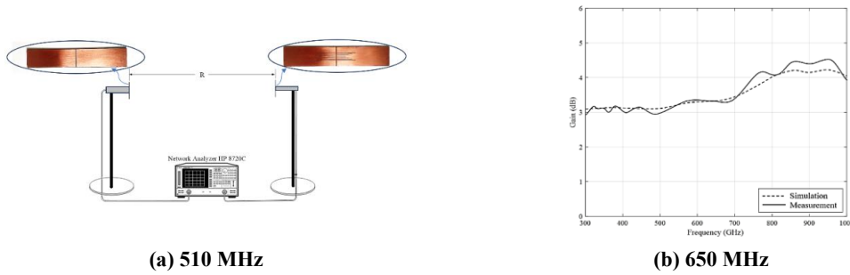
Figure 33. Simulated and measured results of the gain for the 7-slot proposed printed microstrip dipole antenna. (a) Hardware setup to measure the gain, and (b) Gain of the printed dipole antenna.
