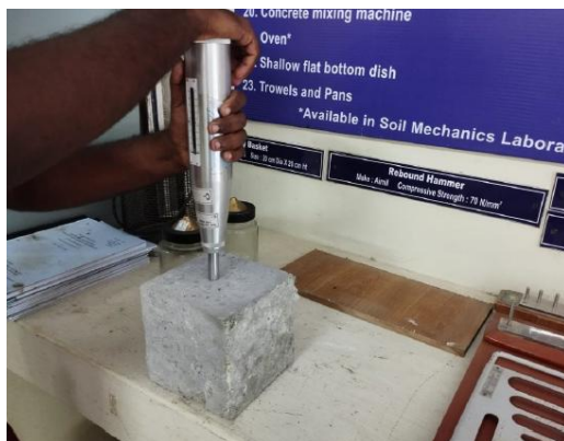
Figure 6. Rebound hammer Test
