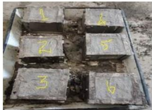
Figure 7. Casting of cube specimens
