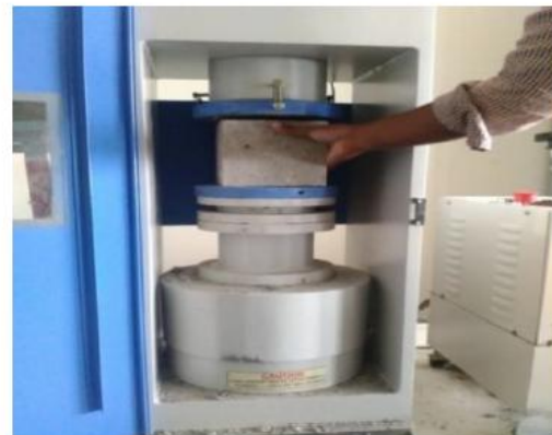
Figure 8. Testing of compressive strength for concrete
