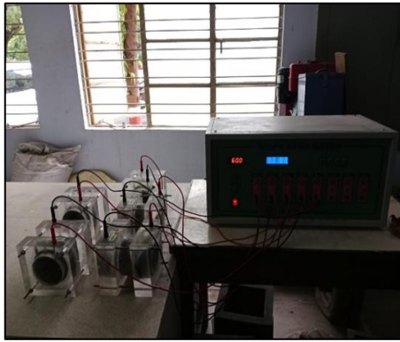
Figure 6. Rapid chloride penetration test setup
