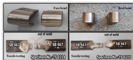
Figure 9. Failed tensile and bend specimens for a welded joint on Cu-Ni alloy
