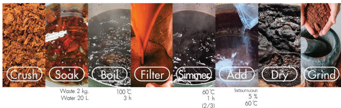
Figure 5 Process of transforming dye extracts into a powdery form
