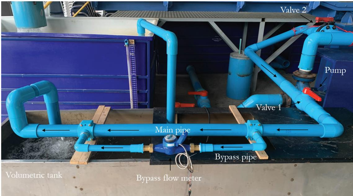
**Figure 3** A flow measurement system setup using a bypass flow meter in a controlled water environment. The system consists of PVC pipes connected in a closed-loop setup, with an inline flow meter installed in the bypass line
