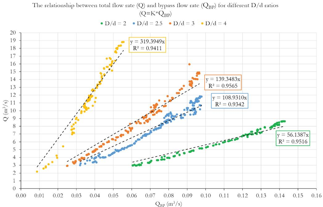
**Figure 4** Test results for determining the K factor of the BPF meter at four D/d ratios
