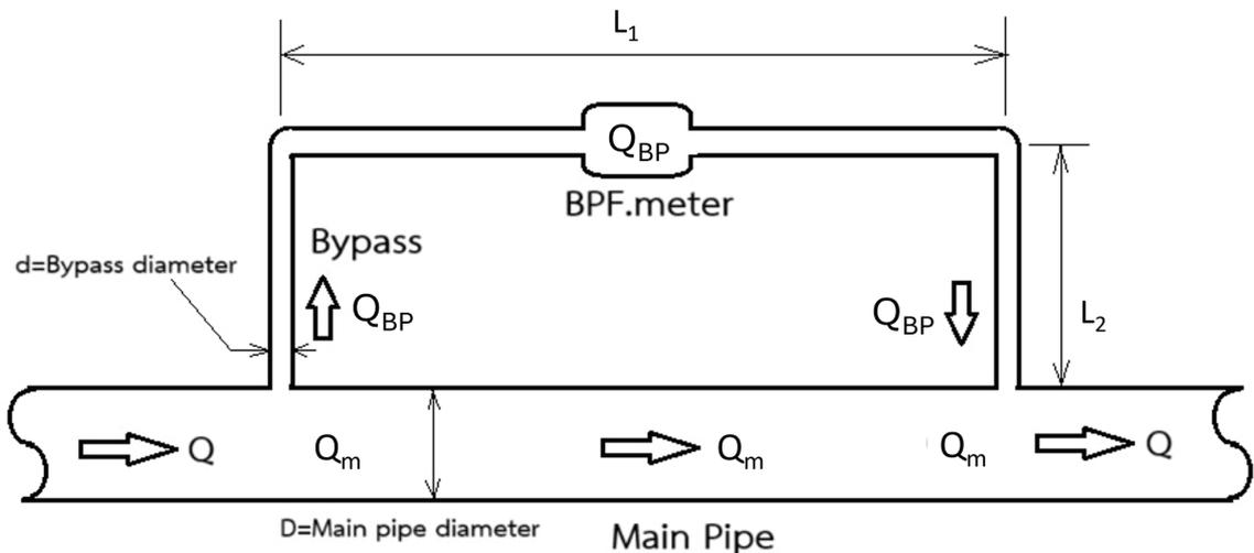
**Figure 1** Top view of a conceptual diagram of the proposed bypass flow meter (BPF meter) system
