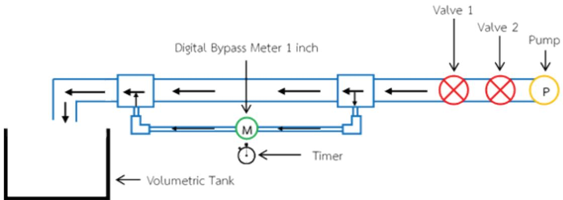
**Figure 2** A conceptual drawing of the proposed bypass flow meter showing the main pipe, the bypass pipe, the control valves, the water meter, the volumetric tank, and the timer, which are integrated into the flow measurement process
