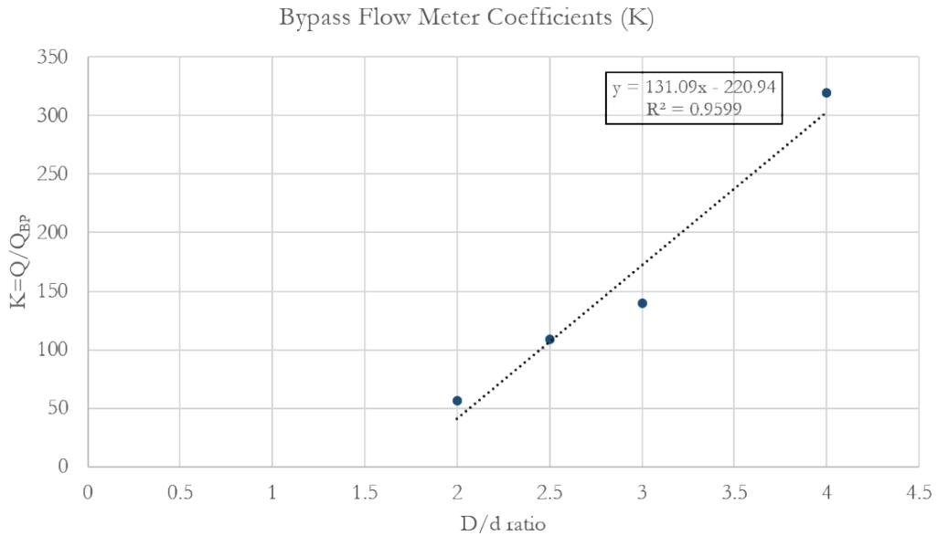
**Figure 5** The relationship between BPF meter coefficient (K) and D/d ratio.
