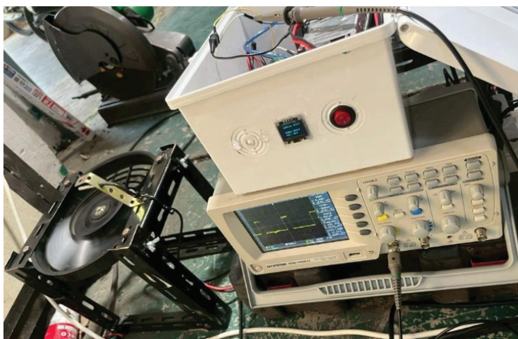
Figure 9 Experimental Setup for PID Tuning and PWM Fan Speed Control Testing
