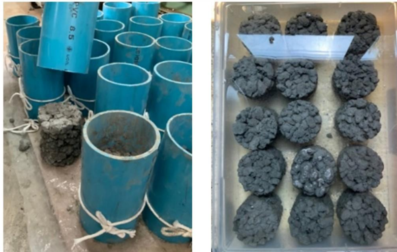
Fig. 2. The as-cast block specimens and the specimens during water curing.
