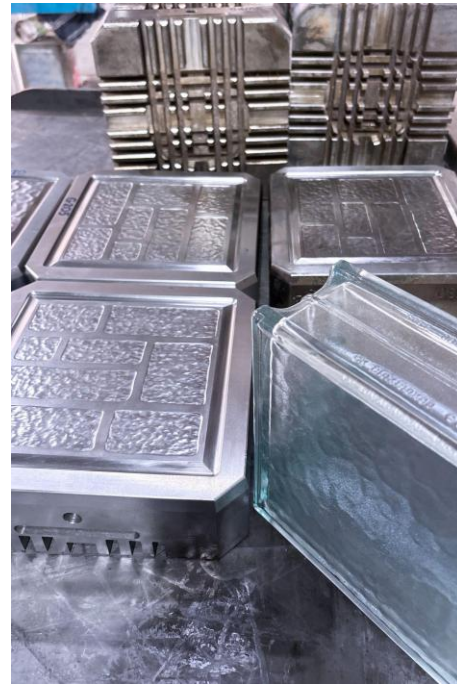
Figure 4. Glass block molds and manufacturing components used in local production processes.
