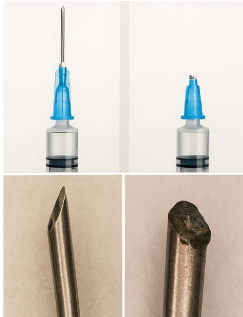
Figure 4 Pre- and post-destruction comparison of syringe needles under macro-optical observation.
