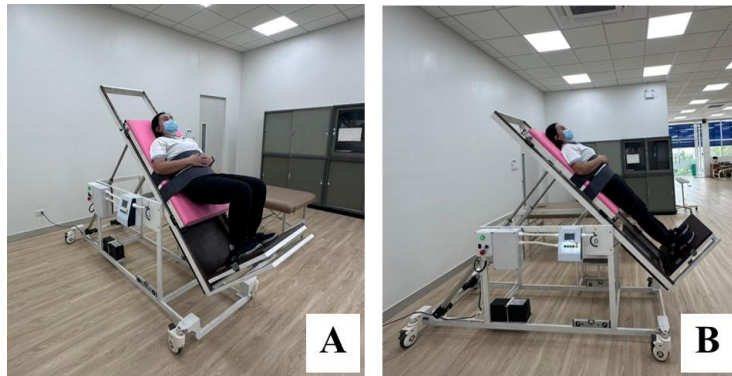
Figure 5 The prototype of an innovative exercise machine for improving lower limb strength: (A) the starting position for exercises using the machine involves flexion of the knee and hip joints; (B) exercises using the machine in knee and hip extension positions are designed to enhance leg muscle function
