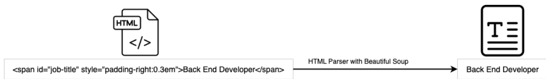
Figure 2 Example of extracting data from HTML structure
